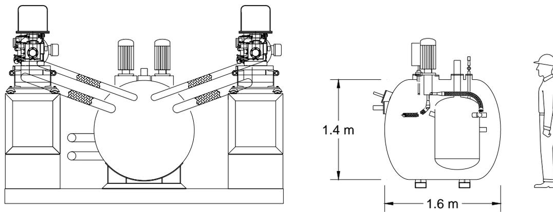
**FIGURE 3.** Scaled mechanical drawing of cold box and skid arrangement
