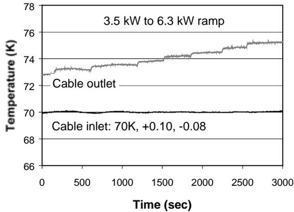
**FIGURE 7.** Ramp response of CRS with cryocooler.
