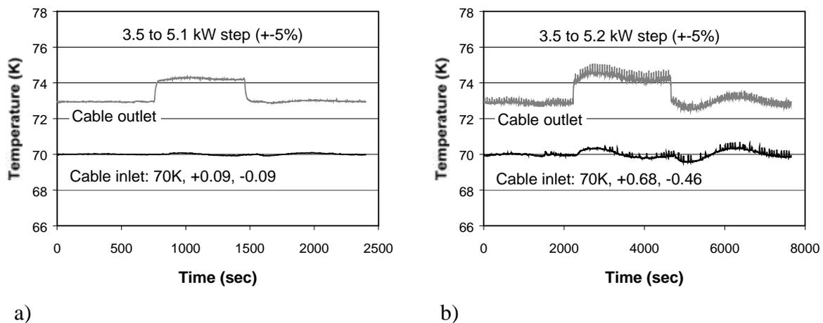
**FIGURE 6.** CRS step control response during cryocooler (a) and vacuum pump (b) operation.
