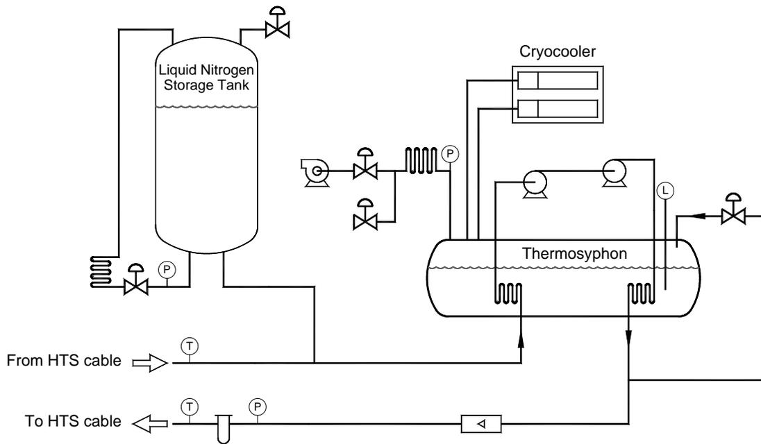
**FIGURE 2.** Simplified schematic of the cryogenic refrigeration system.
