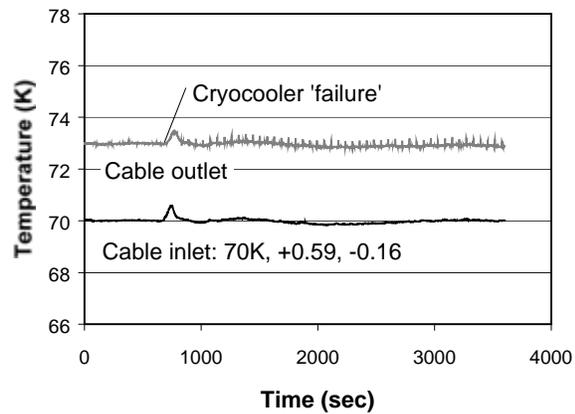
**FIGURE 8.** CRS response to cryocooler failure.
