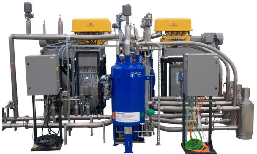
Cooling power available ranges from 500 to over 10 kW at 68K or higher.
